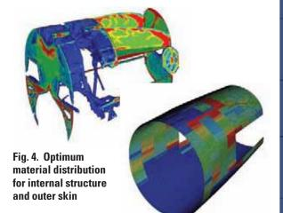
Material distribution was interpreted by experienced engineers from different departments and translated into a CAD design concept. Compared to the A330 design, this new A350 concept features additional shear walls and spatial struts, but fewer frames. The internal load paths, as well as the loadsharing between the structural parts, are significantly different to the A330 concept, resulting in a significant reduction of the internal loads.
